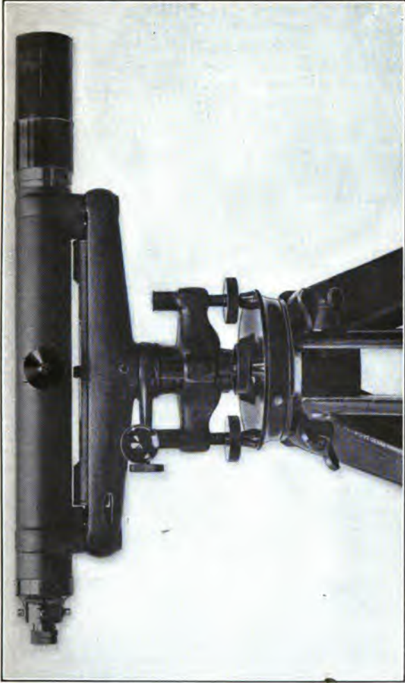
PLATE VI.—ENGINEERS' DUMPY LEVEL (INVERTING EYEPiece). (From a photograph furnished by C. L. Berger & Sons.) (Facing page 80.)
